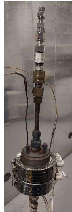
Upper sample vessel with heaters and sample extraction tubes
