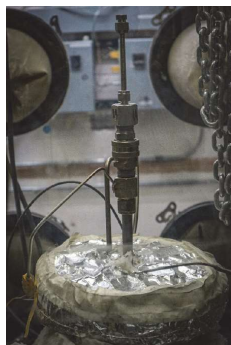
Rapid tube sampler insulated in glovebox
