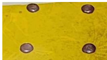
Spotted salt samples for XRF or \mu CAL analysis
